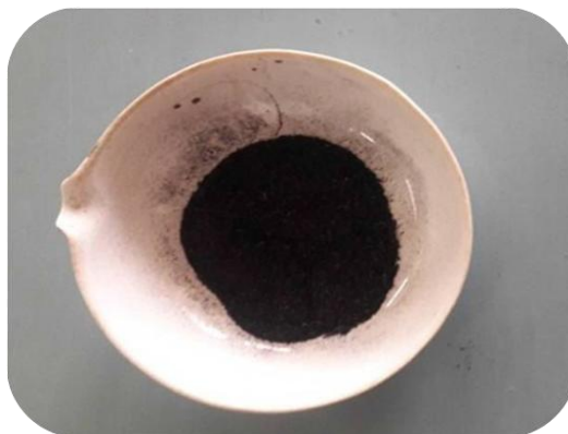
Figure 2. Walnut shell powder heated for 1 hr at 650^\circ C in muffle furnace
